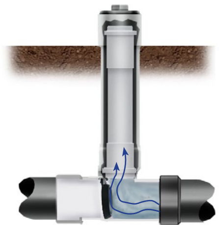
Sewage backflow into building sewer is stopped by flap directing sewage flow into device, building is protected
