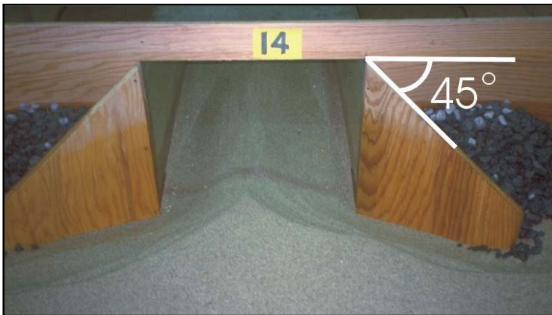
Figure 6.16. Rectangular model with wing walls (FHWA 2003a).
